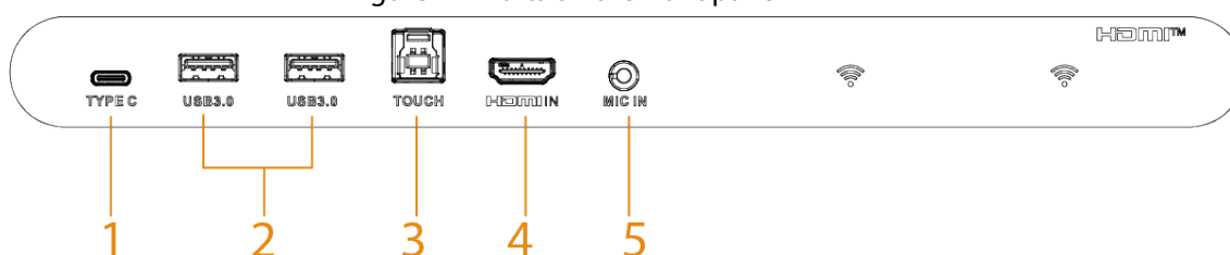
Figure 4-4 Ports on the front panel
